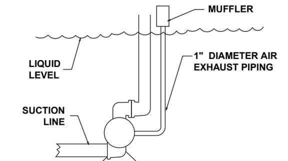
Pump can be submerged if the pump materials of construction are compatible with the liquid being pumped. The air exhaust must be piped above the liquid level. When the pumped product source is at a higher level than the pump (flooded suction condition), pipe the exhaust higher than the product source to prevent siphoning spills.
