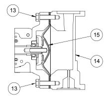
**Diaphragm Orientation** Install diaphragm as shown above.
